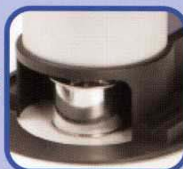
Sample drains automatically
