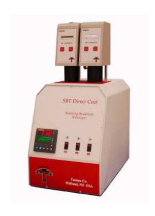
The Scanning Brookfield Technique has always been known for precise technology as evident in the precision of ASTM D5133. Much time has been spent in testing the precision of the SBT Direct Cool unit under a variety of conditions and it has been found to be even more precise than the liquid bath predecessors manufactured from Tannas.
